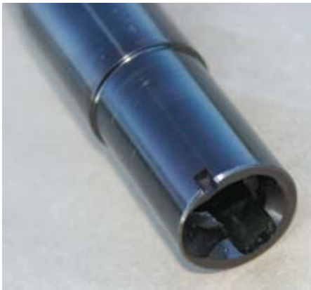
Shank of barrel showing slot that locates barrel inside the receiver ring.
