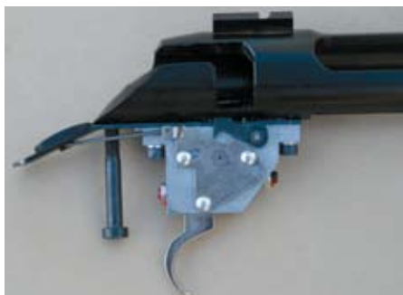
The trigger group and safety catch set-up. The blue tab below the bolt notch is the bolt safety lock.
