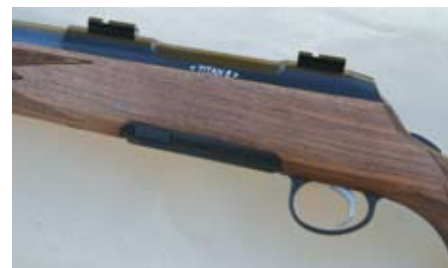
Left side of receiver showing relieved area between the receiver ring and bridge. The rifle is fitted with the small magazine which sits flush with the belly of the stock.
