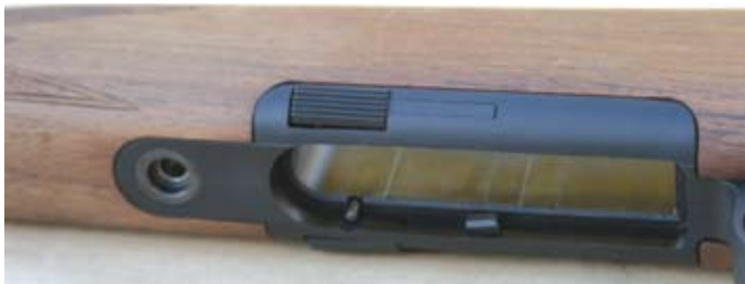
Detail of magazine well and trigger housing showing grooved tab, one retaining catch and the spring-loaded magazine ejector.
