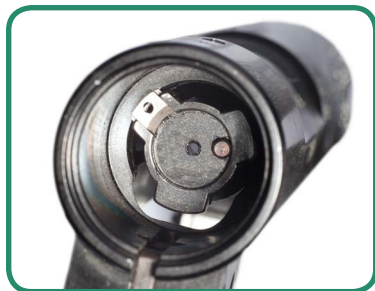
Fig. 10: extractor protrudes over the outside surface of the bolt
