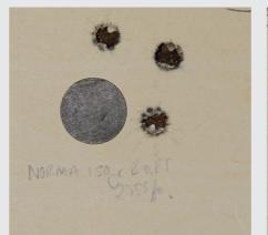
**ABOVE: The Norma 150-gr Ballistic Tips** produced consistent 1.25in groups
