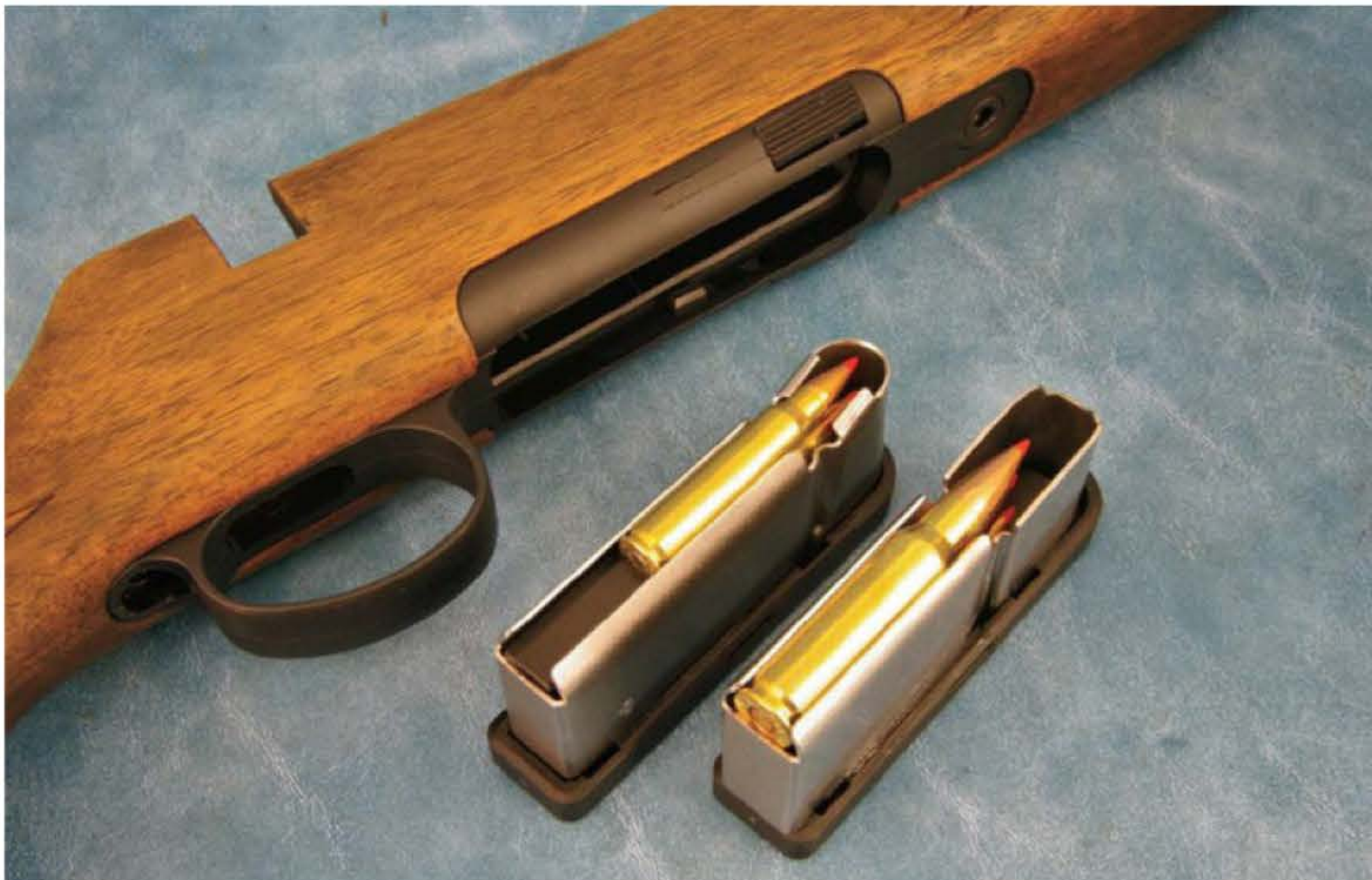
All calibers are based on one receiver length, so standard-length mags are baffled to accommodate shorter cartridges like the .223 and .308 families. They're not the easiest to load.
