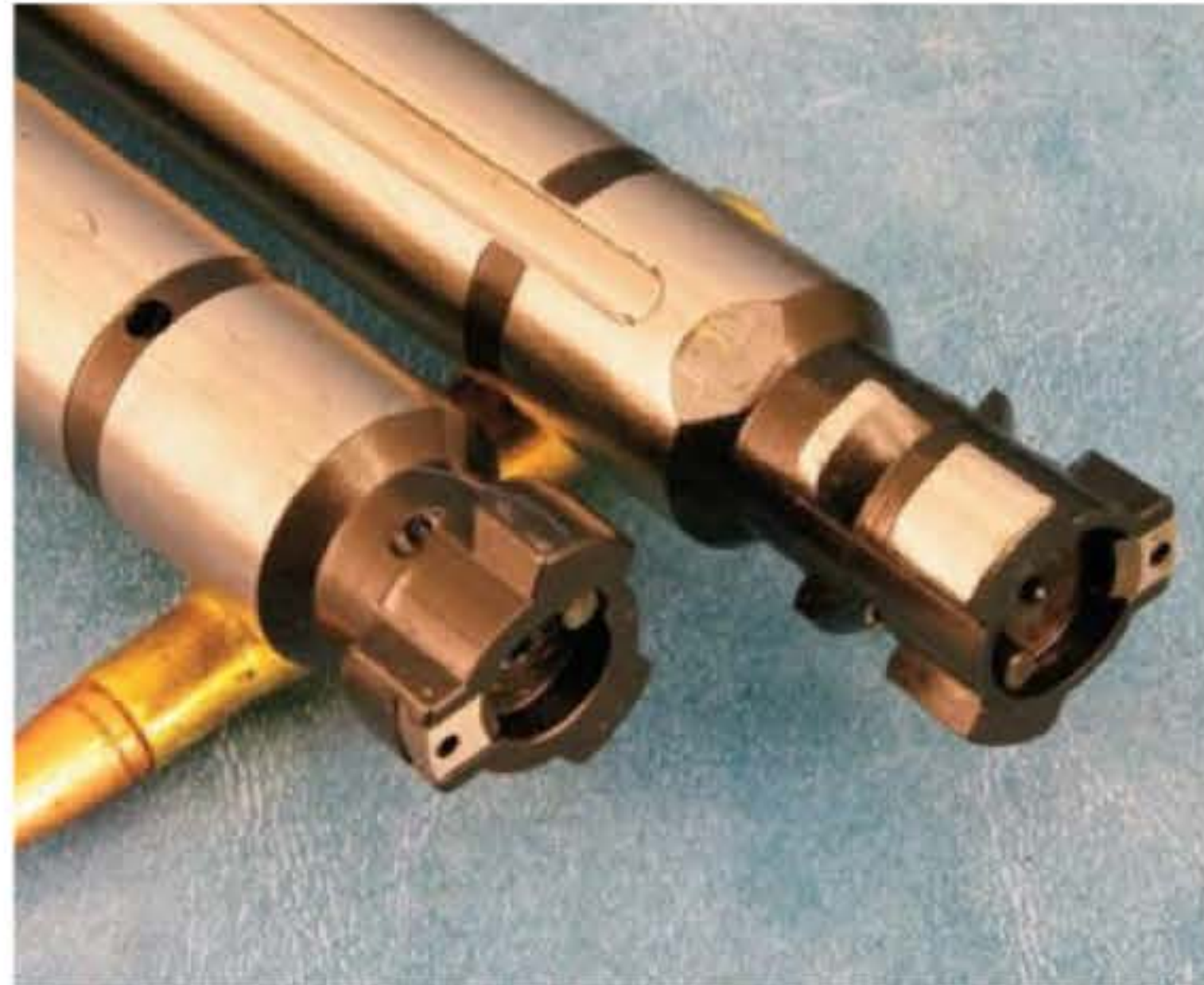
When barreled in .223-size calibers, the bolt is a three-lug affair. In standard and belted magnum calibers there are six locking lugs.
