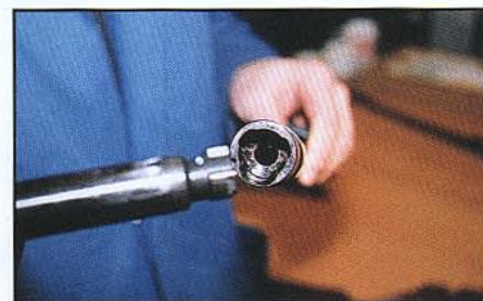
RIGHT: Multiple head lugs lock into recesses in the barrel's breech. The cartridge head is completely encircled by two rings of steel.
